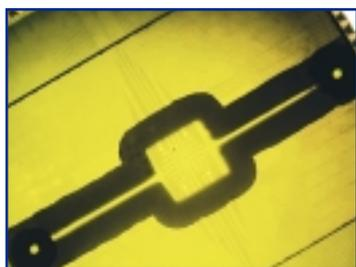
Figura 7 - Fotografia del circuito microfluidico che sormonta il dispositivo a matrice di microelettrodi (Proc. of the Conf. Moems and Miniaturized Systems, part of Spie 2001 International Symposium on Microchining and Microfabrication, M.E. Motamedi, R. Goering (Eds.), 22-25 October 2001, San Francisco, vol. 4561, in press)
