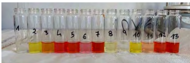
Figure 1 The 13 dyes mixtures used to quantify the sorption from solution where dyes could be simultaneously present.
